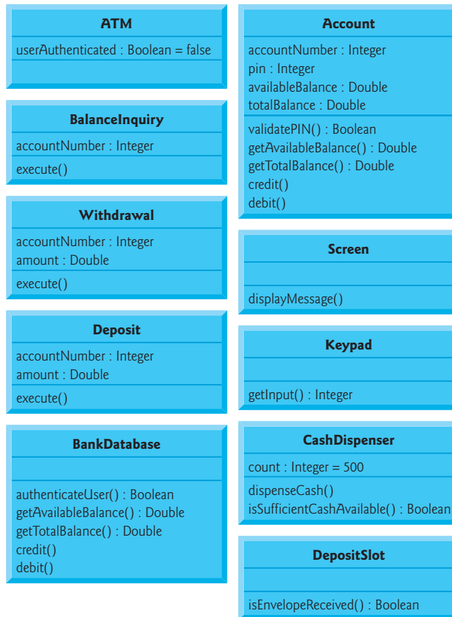
Fig. 25.17 | Classes in the ATM system with attributes and operations.
