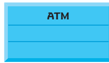
Fig. 25.6 | Representing a class in the UML using a class diagram.
